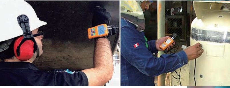
The CTS-30A/ CTS-30B ultrasonic thickness gauge, adopts micro-processor technology and advanced manufacture process design, can do measurement of thickness and acoustic velocity on metal and many different materials.
